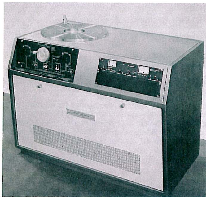
Vacuum pumping system with manual vacuum valve controls and optional vacuum gauge.
