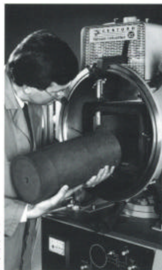
Graphite retort with removable cover is easily installed. With retort removed, furnace is ideal for sintering and other thermal processes.
