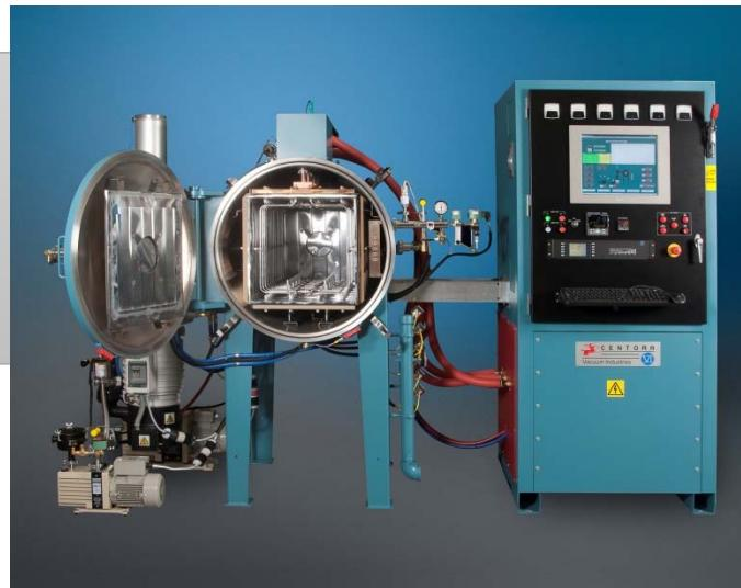
Unlike laboratory or smaller research furnaces, the Workhorse® contains features only found on high-end heat treat furnaces, such as a stainless steel interior vacuum chamber with manual door clamps; heavy duty Molybdenum or Tungsten rod heating elements; and all-metal Tungsten, Molybdenum, or SS radiation shield hot zone for fast heating and cooling, and excellent process cleanliness. You won't find any refractory ceramic insulation or graphite felt/board in this hot zone.
