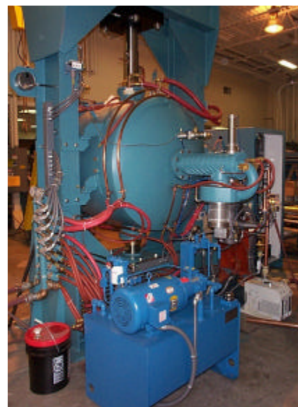
Hydraulic power supply, fan cooling system and diffusion pumping system.
