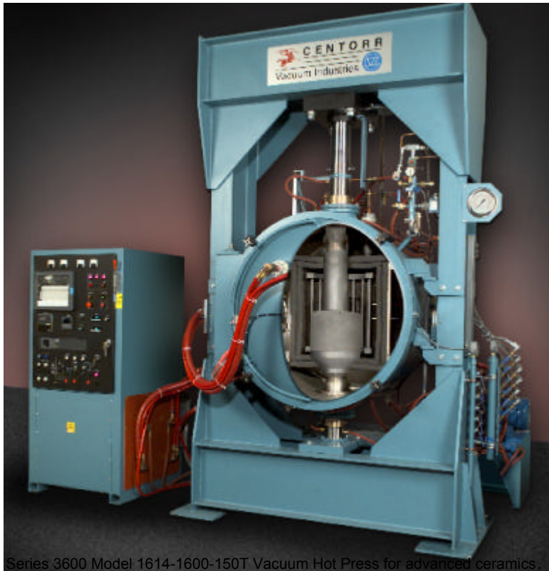
Series 3600 Model 1614-1600-150T Vacuum Hot Press for advanced ceramics
